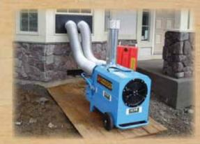
Indirect-fired furnaces are ideal as a temporary heat solution when HVAC is not operable due to lack of permanent power or gas. Heaters have external fuel tanks that can operate up to three days. All of our service vehicles have diesel fuel tanks installed for refueling. Our service includes setup, monitoring, refueling and fuel. Price \$500 - \$700 per week.
